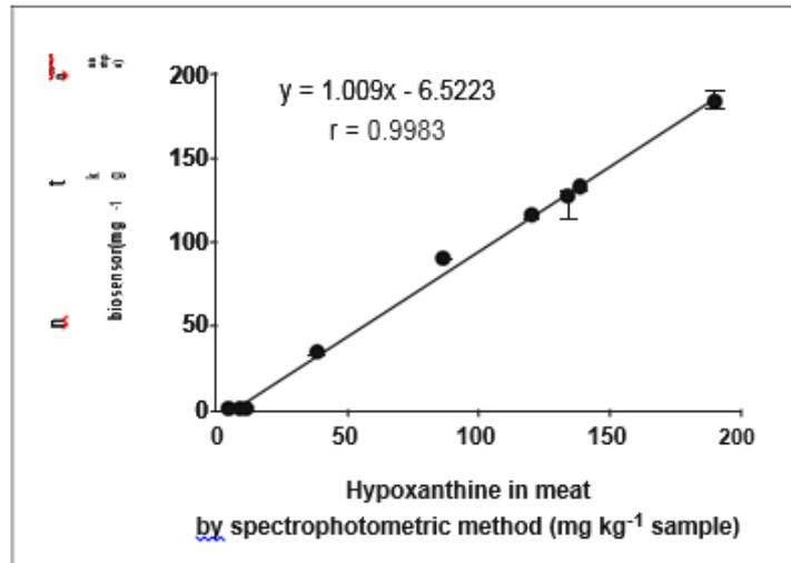
Fig. 6 Correlation curve between hypoxanthine concentrations as detected by standard spectrophotometric (X-axis) method and the present  $\mu$ PAD biosensor (Y-axis)
