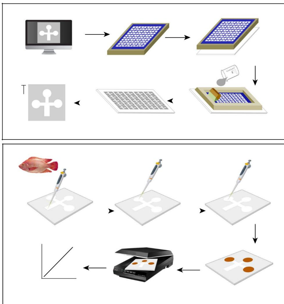
Fig. 1 a Schematic diagram of screen-printing for fabrication of  $\mu$ PAD biosensor and b schematic diagram of colorimetric assay of hypoxanthine on a  $\mu$ PAD biosensor
