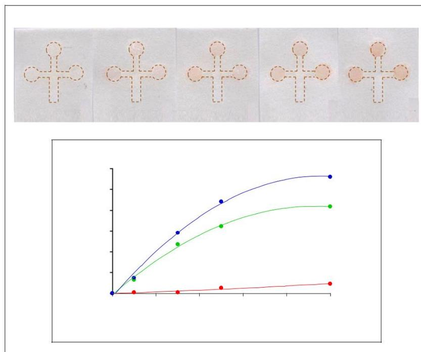
Fig. 2 a Color change in the  $\mu$ PAD biosensor using various concentrations of hypoxanthine from 0 to 100 mg L<sup>-1</sup> and b RGB intensity values results
