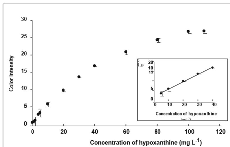
Fig. 4 Calibration curve for hypoxanthine under optimal conditions. Inset: Linear range of the calibration curve for 5–40 mg L<sup>-1</sup>
