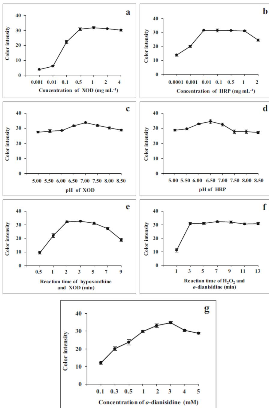
Fig. 3 Optimum conditions of hypoxanthine detection using the  $\mu$  PAD biosensor device. a Concentration of XOD. b Concentration of HRP. c Effect of pH value of XOD. d Effect of pH value of HRP. e Reaction time of hypoxanthine reacting with XOD. f Reaction time of H<sub>2</sub>O<sub>2</sub> reacting with o-dianisidine. g Concentration of o-dianisidine
